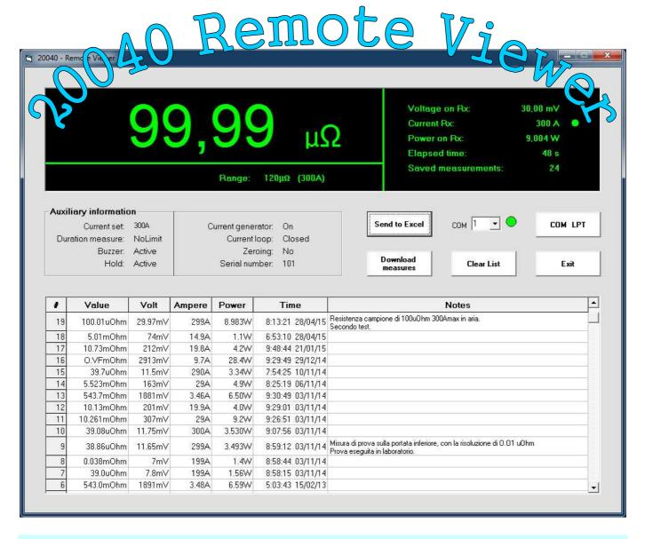
**20040 Remote Viewer** is a software for Windows that allows you to remotely view the resistance measurement, auxiliary measures, settings, and other alerts. Also you can download the data stored in non-volatile memory of the instrument, each consisting of: resistance, voltage on Rx, the actual current through Rx, the power dissipation on it, the date and time of the recording and finally notes associated with the measures, where present.
